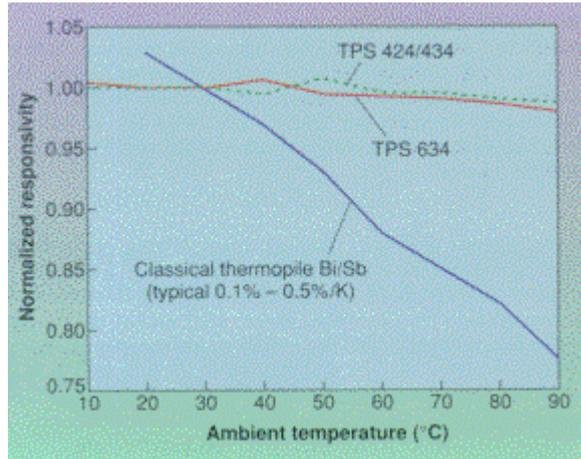
**Figure 3. Thermopiles made using polysilicon and aluminum as thermoelectric materials exhibit low temperature-dependency sensitivity when compared to conventional Bi/Sb devices.**
