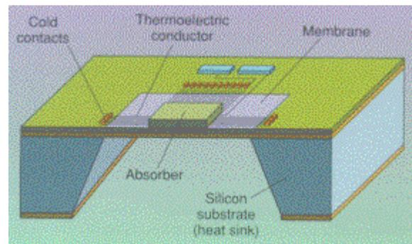
**Figure 1. Standard photolithographic techniques etch a silicon substrate to create a silicon-based thermopile sensor chip. Cutaway view reveals the IR-sensing area in the middle of the substrate on a 1- $\mu$ m thick membrane of SiO<sub>2</sub>/Si<sub>3</sub>N<sub>4</sub>.**
