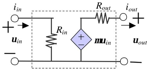
$$R_{in}=10\text{k}\Omega, m=100, R_{out}=10\Omega$$
