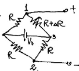
先求 open-circuit voltage  $V_{oc}$
